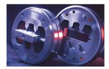
An extruding tool is completely processed within **a few minutes**. According to the processing time, surface values of Ra 0.2 µm and Rz 1 µm are obtained.
