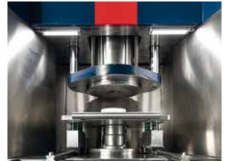
The fixed diameter of the medium cylinder (75 – 250 mm) can be reduced easily within a short conversion time by using one or more reduction kits (optional).
